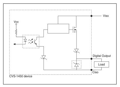
Figure 4-6. Example of Connecting an Isolated Output to an External Load
